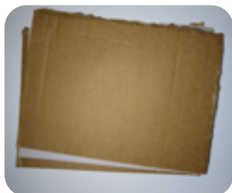
Cardboard sandwiching the specimen
